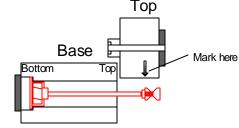
2. Mount the Base tenon into the chuck and insert the Top into the Base. Bring the tailstock up to the Top (a small cone helps centerin the hole) and tighten so that the Base and Top are friction fit. Turn the peppermill to shape as desired.
