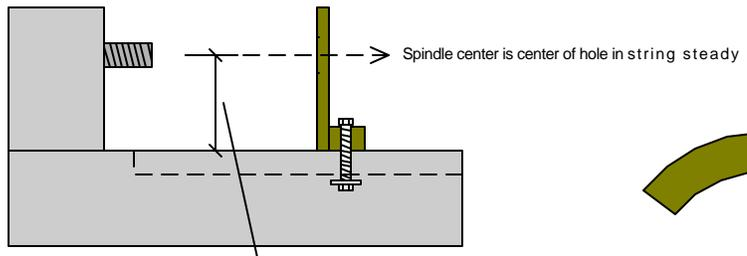
Distance from bed to center of spindle
